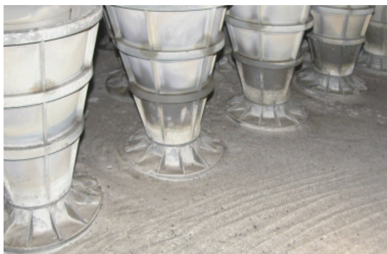
Flue gas scrubber before the treatment with FINEAMIN HELAWAX®
